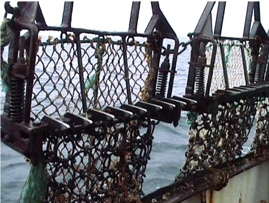
Left, close-up of the seabed-penetrating teeth on the cutting bar of a Newhaven pattern scallop dredge., which is typically dragged along the seabed for hundreds of metres at around 2.5 knots (3 mph, 1.3 m/s).
